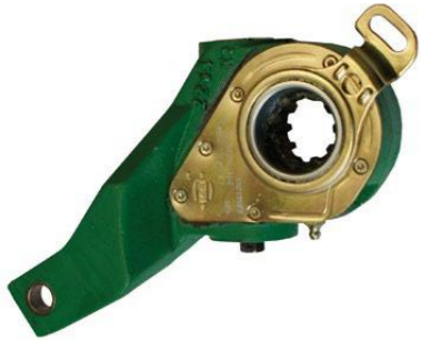
Fren Ayar Kolu 4V2020 Daf Slack Adjuster 4V2020 Daf
