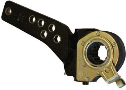
Fren Ayar Kolu 6Y1515 Treyler Slack Adjuster 6Y1515 Trailer
